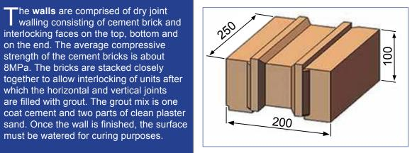
Solbric interlocking cement brick detail
