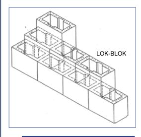
A & D Holdings external wall interlocking blocks detail
